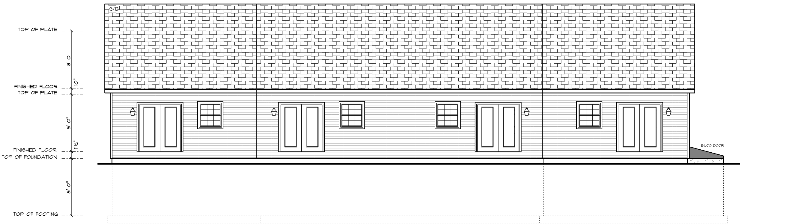
REAR ELEVATION SCALE 1/4" = 1'
